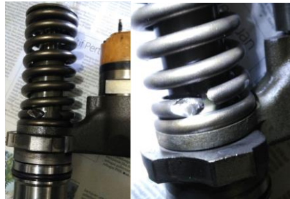
Figure 2. Spring injector broken
