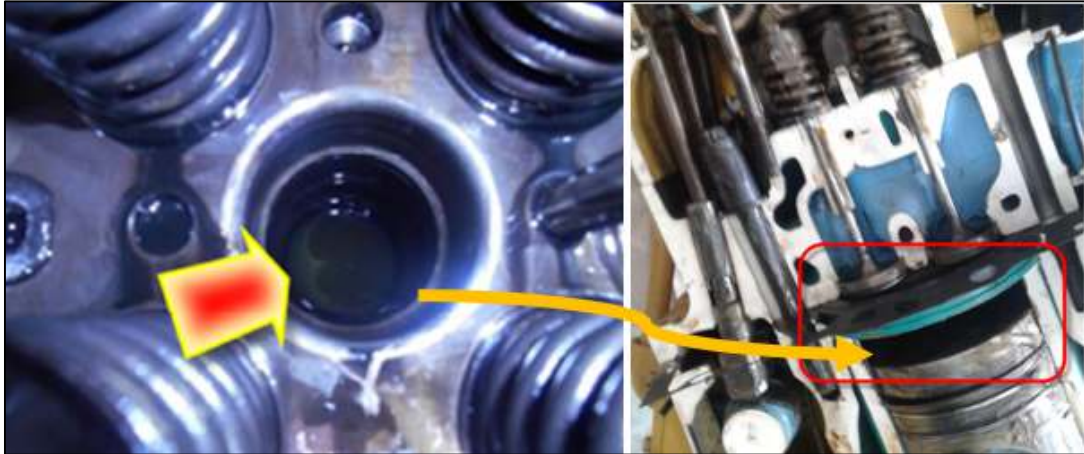
Figure 2. Solar is in the combustion chamber.
