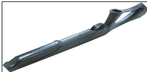
Figure 3. Original ABS trial material plus 50% recycled material and 2.5% synthetic fiber
