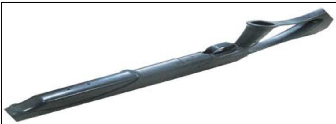
Figure 1. The original 100% ABS trial material without additional of synthetic fiber.
