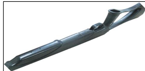
Figure 4. Original ABS trial material plus 50% recycled material and 2.5% synthetic fiber.
