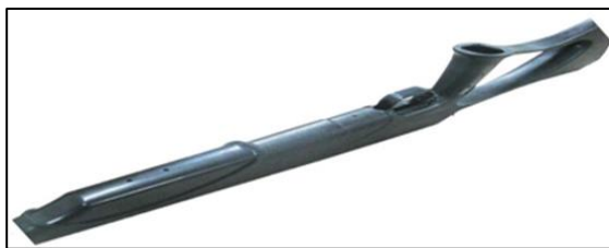
Figure 1. The original 100% ABS trial material without additional of synthetic fiber.
