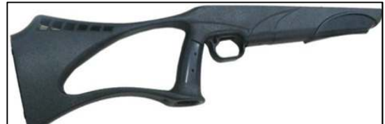
Figure 2. Product original trial material ABS plus 10% recycled material from original material weight without additional of synthetic fiber
